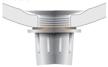
We recommend the installation of a flexible closure between lower edge of the urinal drain and the Adapter-key. The Adapter-Key was designed to be tightened by hand without the help of other tools.
