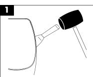
**USE UTILITY KNIFE TO CUT CAULK** then use a putty knife and mallet to remove the bowl. Remove hanger brackets, scrape off caulk, and clean the wall.
