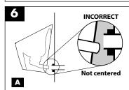
A. Hang the bowl on the bracket and check tail pipe alignment, then remove the bowl and adjust the bracket as needed.
