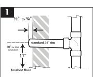
SET DRAIN LINE HEIGHT 17" from finished floor (standard 24" rim) or 10" for ADA installation. Threaded nipple should extend ½ to ¾" from wall.
