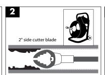
**IMPORTANT:** Use a drain machine to remove build-up inside pipes. Clean up to 25 feet deep then flush with water to remove cutting debris. Never install on copper DWV.
