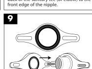
PLACE THE SEAL INTO THE FLANGE with the ribs facing out. Install the flange with washers and hex nuts, but do not tighten completely.
