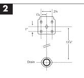
**CARRIER STUD PLACEMENT If using** in-wall carrier, set bearing rods as shown above.
