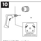
DRILL HOLES with 5/16" masonry bit for the lower anchor screws and insert plastic anchors.
