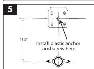
MEASURE & MARK THE ROUGH-IN if in-wall carrier is not used. Use a 5/16" masonry bit to drill hole, then install the hanger bracket with one plastic anchor and screw.
