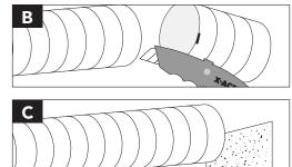
**B.Cut the tube** at the groove using a sharp utility knife to ensure a square, flat cut.
