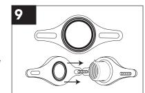
PLACE THE SEAL INTO THE FLANGE with the ribs facing out. Install the flange with washers and hex nuts, but
