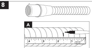
**A. Find the drain nipple depth** on the Tube Cutting Chart (left). **Measure and mark the specified trim length** on the insert tube at the nearest 1/4" groove.
