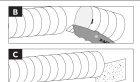
**B.Cut the tube** at the groove using a sharp utility knife to ensure a square, flat cut. C.Clean burrs from the cut end by using
