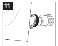
HANG THE BOWL, inserting tailpipe into bushing, then install anchor screws with washers.
