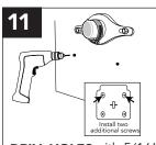
**DRILL HOLES** with 5/16" masonry bit for the lower anchor screws and mounting plate and insert plastic anchors where indicated.
