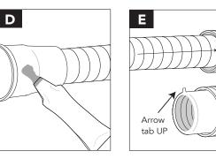
**D. Apply lubricant** to the outside of the rubber bushing and ribbed inside area.
