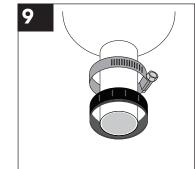
PLACE THE HOSE CLAMP and compression nut onto the housing tailpipe.
