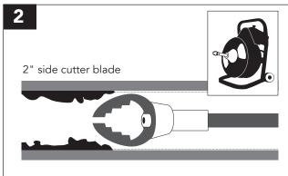
**IMPORTANT:** Use a drain machine to remove build-up inside pipes. Clean up to 25 feet deep then flush with water to remove cutting debris. Never install on copper DWV.
