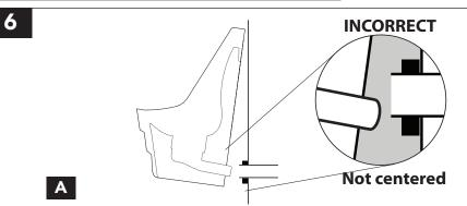
A. Hang the bowl on the bracket and check tail pipe alignment, then remove the bowl and adjust the bracket as needed. Re-hang and re-check bowl alignment with the drain line. Tail pipe should align with center of drain line.
