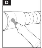
**D. Apply lubricant** to the outside of the rubber bushing and ribbed inside area.
