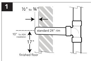
**SET DRAIN LINE HEIGHT** 17" from finished floor (standard 24" rim) or 10" for ADA installation. Threaded nipple should extend ½ to ¾" from wall.
