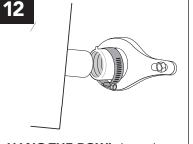
**HANG THE BOWL,** inserting tailpipe into bushing, then install anchor screws with washers. TIGHTEN FLANGE **BOLTS AND HOSE CLAMP.**
