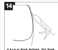
**CAULK THE BOWL TO THE WALL** if there is good flow and no leaks or standing water.
