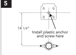
MEASURE & MARK THE ROUGH-IN is in-wall carrier is not used. Use a 5/16" masonry bit to drill hole, then install the hanger bracket with one plastic anchor and screw.
