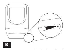
**B. Mark anchor holes** then remove bowl without moving hanger bracket.
