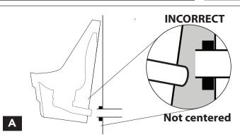
**A.Hang the bowl on the bracket** and check tail pipe alignment, then remove the bowl and adjust the bracket as needed. **Re-hang and re-check bowl** alignment with the drain line. Tail pipe should align with center of drain line.
