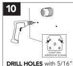
masonry bit for the lower anchor screws and mounting plate and insert plastic anchors where indicated.
