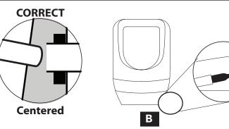
B. Mark anchor holes then remove bowl without moving hanger bracket.
