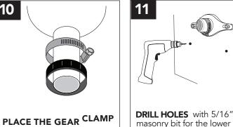
masonry bit for the lower anchor screws and insert plastic anchors.
