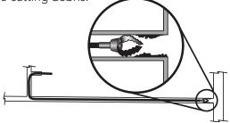
• Drain pipes should also have proper slope, to allow complete drainage of liquid through the piping system after each use.
