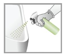
Activate the new HPKV by flushing about 5 liters of soapy water. Spray urinal with pH neutral cleaner\*. Do NOT wipe afterwards.
