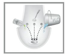
Flush the urinal with a bucket of water container cleaner, scrub thoroughly with a brush and then flush with a bucket of water containing cleaner again.
