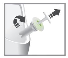
Place the Service- Key into the High Performance Key-Valve (HPKV) and turn counter clockwise to unscrew the HPKV from the Key-Adapter
