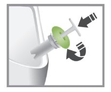
Using the Service-Key, screw the HPKV clockwise into the Key-Adapter until the valve sits evenly.
