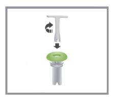
Remove HPKV from packaging and, with a slight counter clockwise twist, plug they Service-Key into the new HPKV cartridge.
